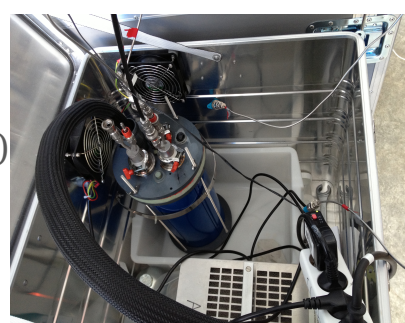
-60° C drying system, with Mg(ClO 4 ) 2 trap follow-up
